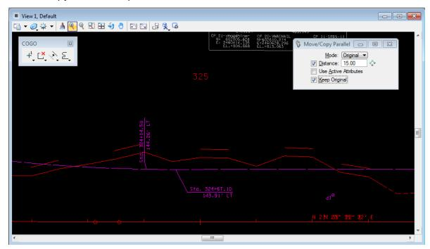
Now use MicroStation's **Smart Line** tool with sharp breaks to set a preliminary proposed R.O.W. line.
