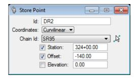
The station & offset should be locked in. Data point in the view to store the point **DR2**.
