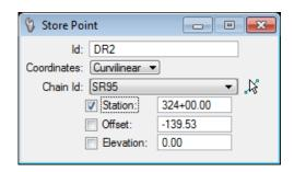
Now **go down** to the **Offset** and round to the nearest even foot which should be about **-140**. Don't forget the negative sign since we are on the left side of the road.
