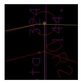
**10)** Repeat step 9 to store point **DR3** at Station **327+00**, Offset **-130**. You must click on the lock toggle boxes to un-lock the station and offset values and return to dynamic location mode.
