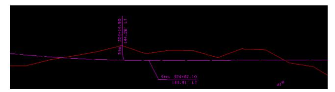
3) Open up D&C Manager and select item Drafting Standards → Prop. R.O.W.→ R.O.W. Prop. In the secondary dialog, click on the Draw Plan & Profile button. Set the dialog to chains and single click on our proposed R.O.W. chain DROW1. Linework and distance/bearing annotation is placed.
